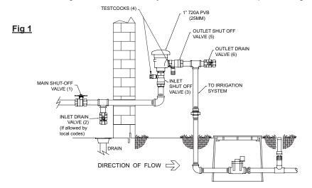
The discharge should cease by the time the shut-off valve is in the full open position.
