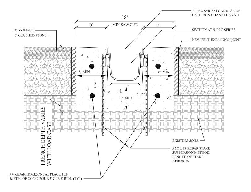
• CHANNELS TO BE INSTALLED WITH GRATE. GRATE TO BE PROTECTED FROM CONCRETE POUR.
