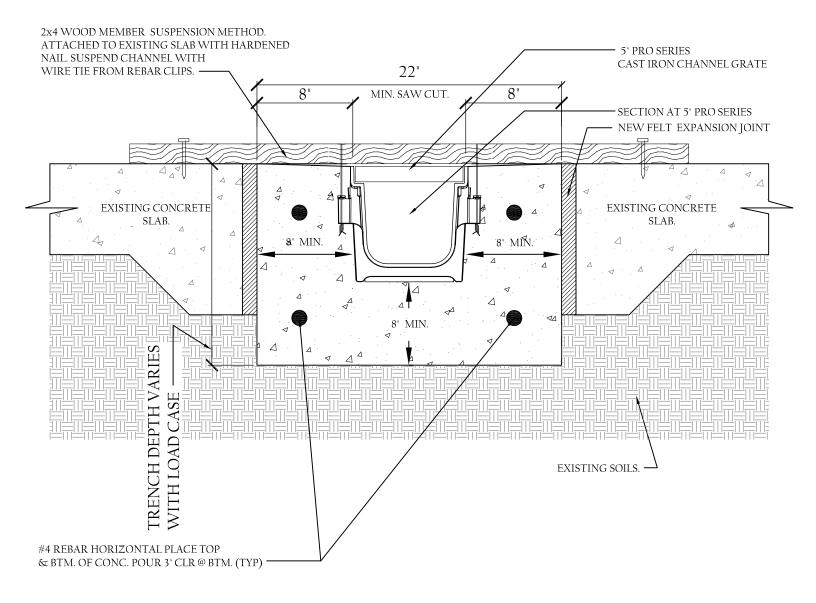
• CHANNELS TO BE INSTALLED WITH GRATE. GRATE TO BE PROTECTED FROM CONCRETE POUR.
