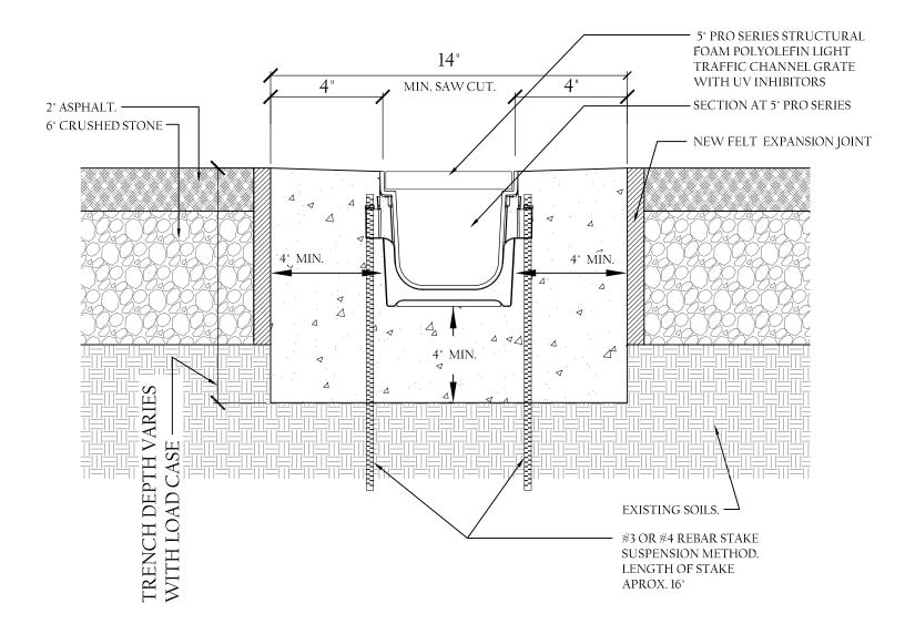
• CHANNELS TO BE INSTALLED WITH GRATE. GRATE TO BE PROTECTED FROM CONCRETE POUR.
