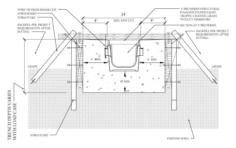
• CHANNELS TO BE INSTALLED WITH GRATE. GRATE TO BE PROTECTED FROM CONCRETE POUR.
