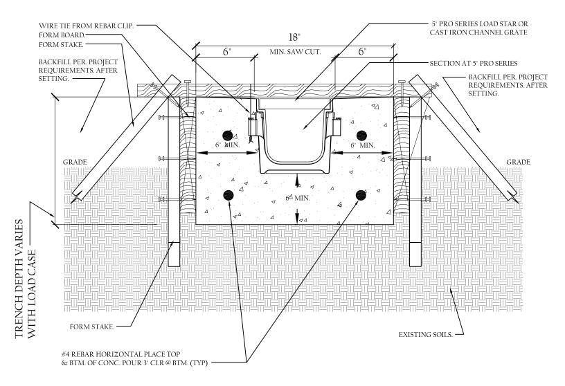
• CHANNELS TO BE INSTALLED WITH GRATE. GRATE TO BE PROTECTED FROM CONCRETE POUR.
