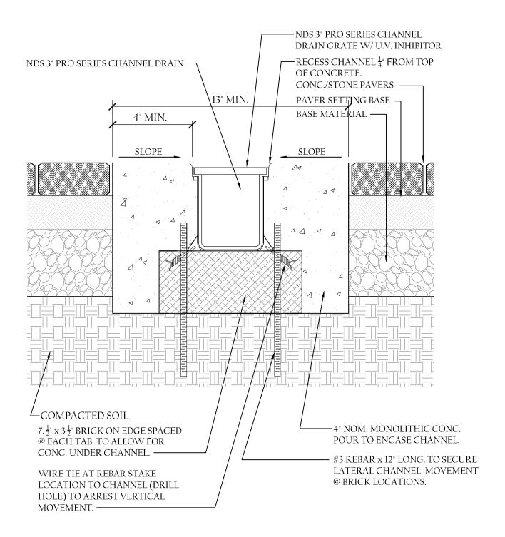
CHANNELS TO BE INSTALLED WITH GRATE. GRATE TO BE PROTECTED FROM CONCRETE POUR.
