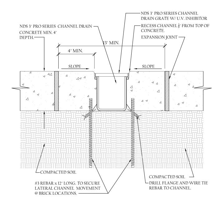
CHANNELS TO BE INSTALLED WITH GRATE. GRATE TO BE PROTECTED FROM CONCRETE POUR.
