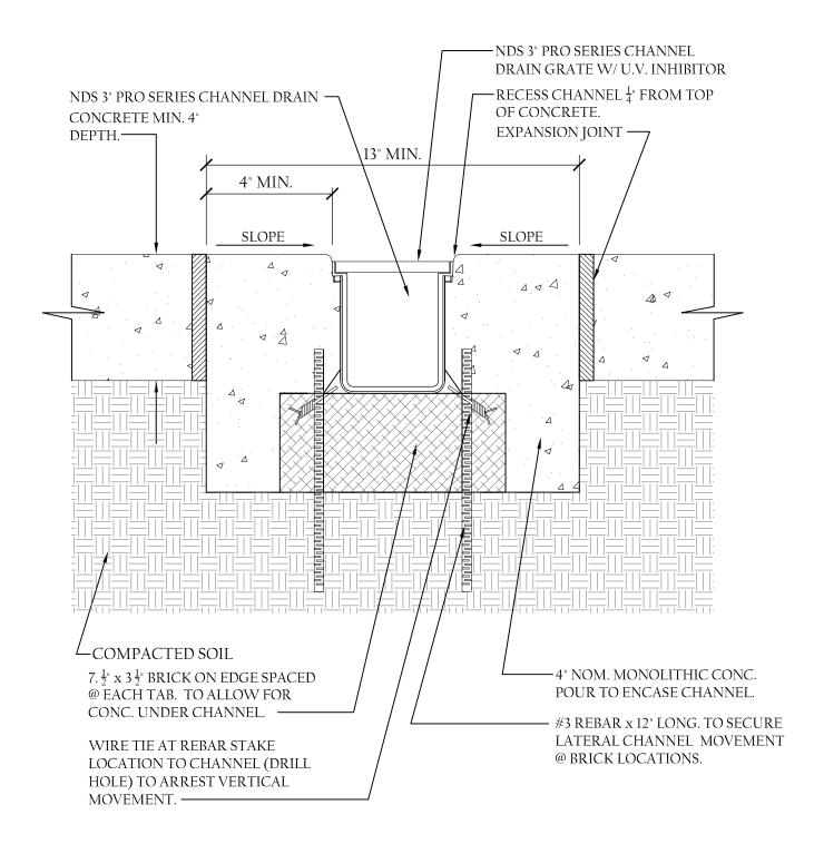
• CHANNELS TO BE INSTALLED WITH GRATE. GRATE TO BE PROTECTED FROM CONCRETE POUR.
