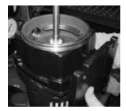
4. Apply rubber lubricant to the seal ID. Install seal assembly onto motor shaft.
