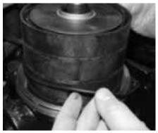
10. Install outer sleeve onto o-ring, positioned so that seam is down.
