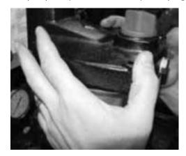
13. Install a lock washer on each bolt. Insert bolts into bracket. Install lock nuts and tighten evenly to 17-19 ft/lbs.
