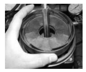
7. Install impeller with metal eye ring up.
