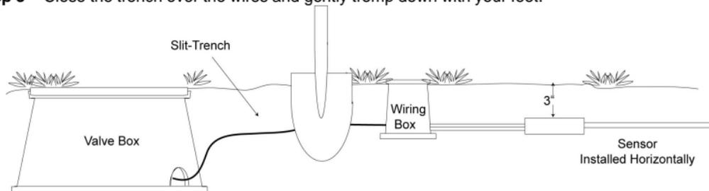
**Before connecting any wiring place the controller in OFF mode by depressing the power button.** Each valve has two wires. You will use these two wires and the three from the sensor to make three connections. Use only direct burial or other water-proof connectors to make these connections.
