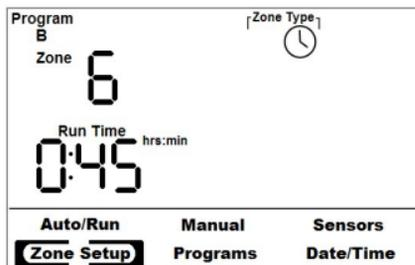
**Step 4. Edit Run Time:** The run time flashes. Press + or - to adjust. Hold the + or - button to accelerate. "OFF" occurs at zero minutes, and disables watering of that zone for the selected program.
