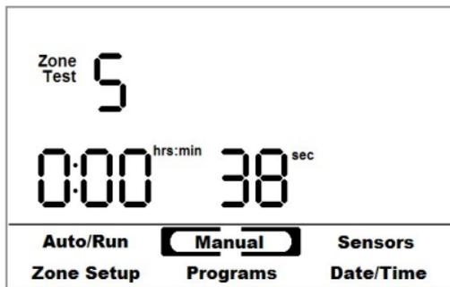
Use this option to water a zone for a specific duration. Use + or – to select the zone number to water, then press Enter. Use +/- to set the desired watering duration, then press enter again to start watering that zone. The controller will switch to the Auto/Run screen to show the watering activity. Press cancel to stop all manual watering.
