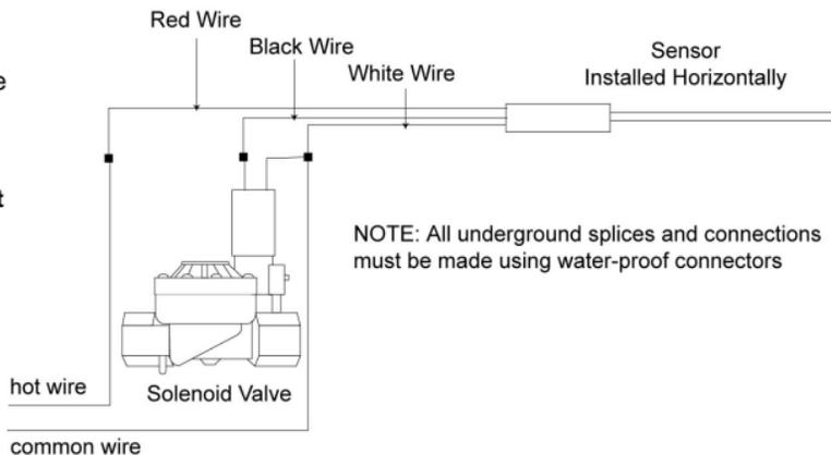
Making an underground connection using the supplied direct burial connectors.
