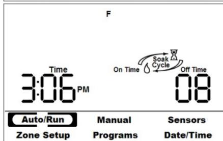
When a zone is soaking and no other watering activity is pending the controller will display the current time and a count down of the soaking time.
